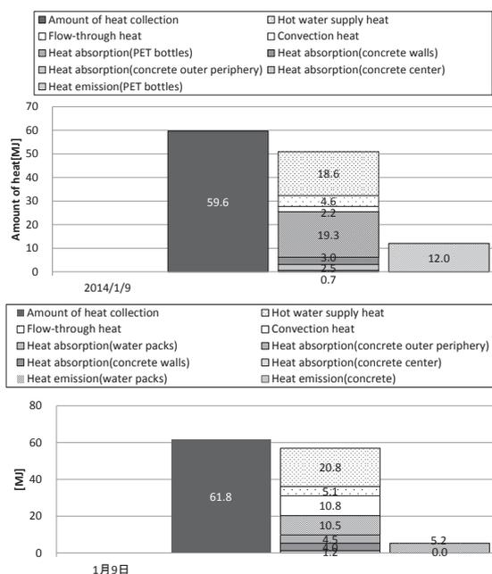
Figure 2. heat balance in the underfloor (Experiment 4)
